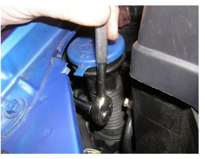
You can get a bit more room to work by unscrewing the washer bottle filler pipe but be sure to stuff a rag into the hole in case you drop the nut or worse still the ratchet. ( I only just thought of that, I didn't do it at the time!!!)
