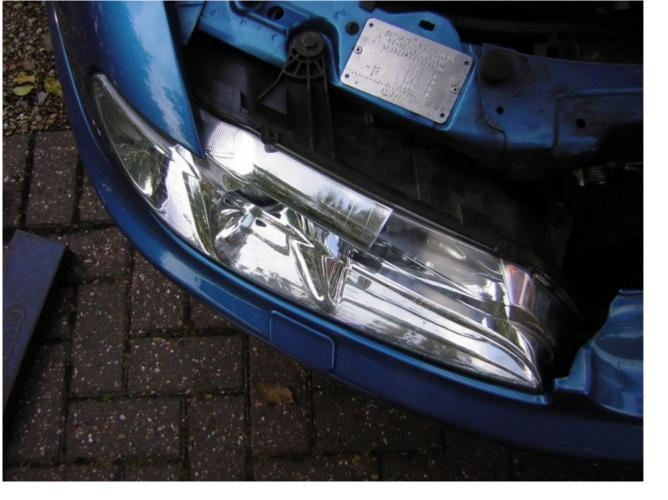
A quick test of the lights showed the main beam hotspots to be better placed than before but I need to do a proper check on the dip beams to make sure the offside one is not blinding anyone. I also levelled the beams up using an allen key in the RH adjuster.
