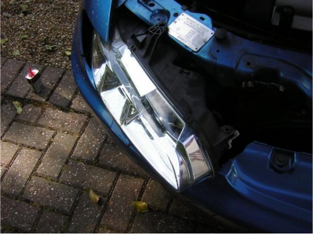
Also it helped to twist the levelling motor about 1/4 of a turn (I didn't need to take it right off). After some fiddling about the light came off in my hand!! It was then possible to get a good look at the two hidden mounting studs and the appropriate lugs on the headlight.
